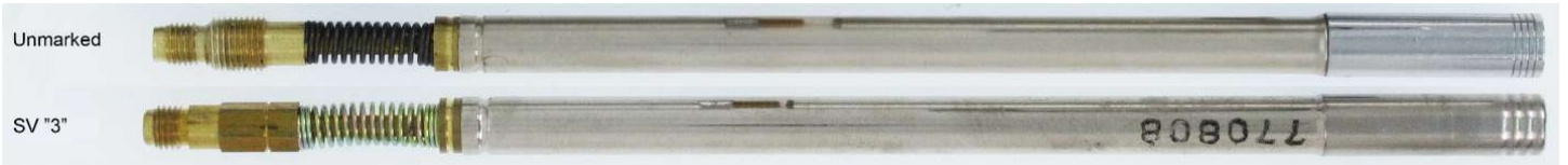
Image 14: Differences between internal Unmarked SV and "3" SV
